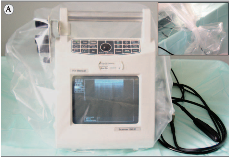
Figure 2: Ultrasound machines showing three different types of covering to prevent dust entering the machine, but with the cables and transducers uncovered in each case. A: Falco Vet 100 (Esaote-Pie Medical, Maastricht, The Netherlands) completely covered with a transparent disposable plastic bag, closed at the end with a plastic strip (insert); B: HS 1201 (Honda Electronics Co Ltd, Tokyo, Japan) completely covered with polyethylene wrap (household cling-film); C: HS 1201 incompletely covered with a transparent disposable plastic bag open at the end (insert).
