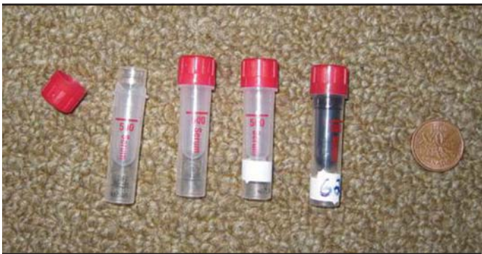
Figure 1: Label the 500- \mu L serum collection vial with a pre-glued paper label.
