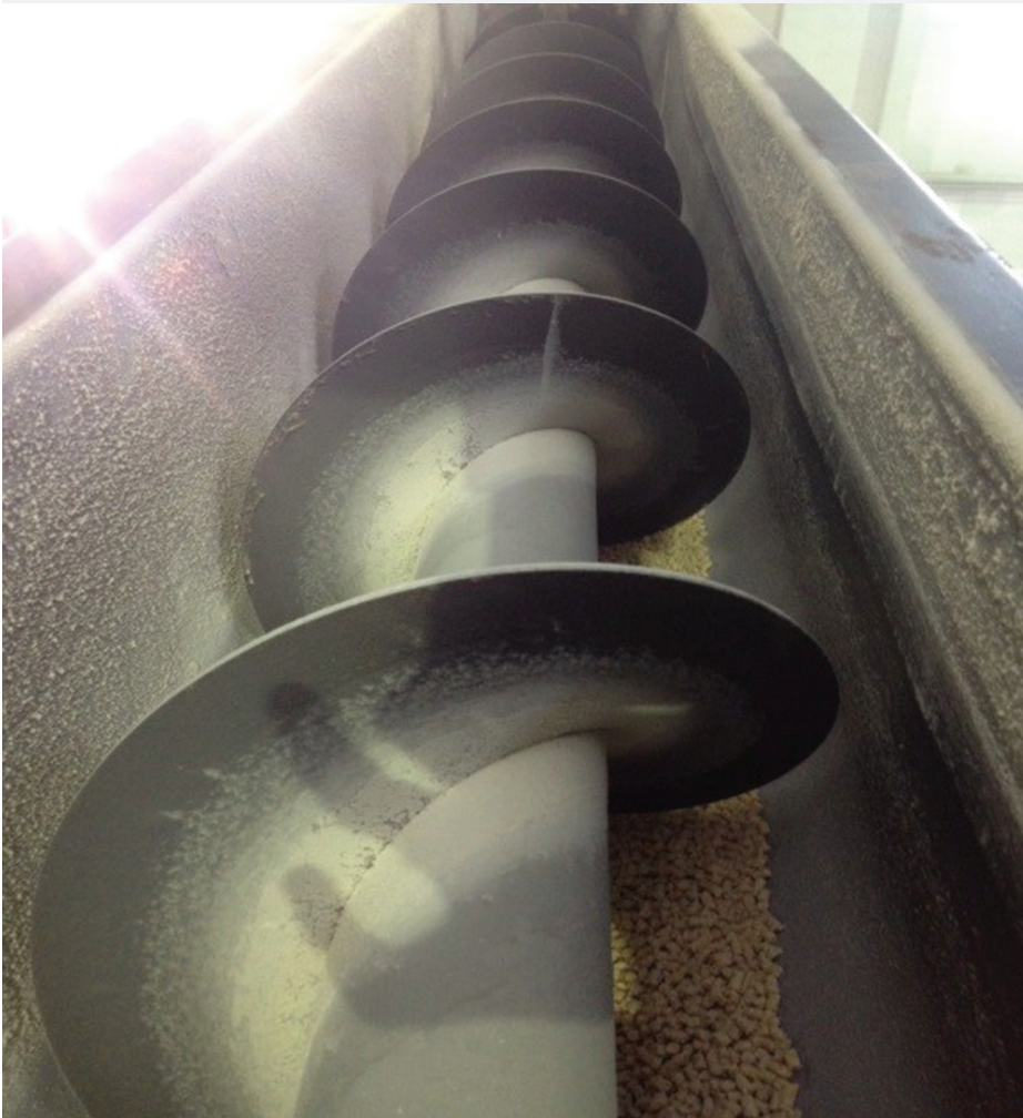
Figure 5: Screw conveyor with potential contamination
