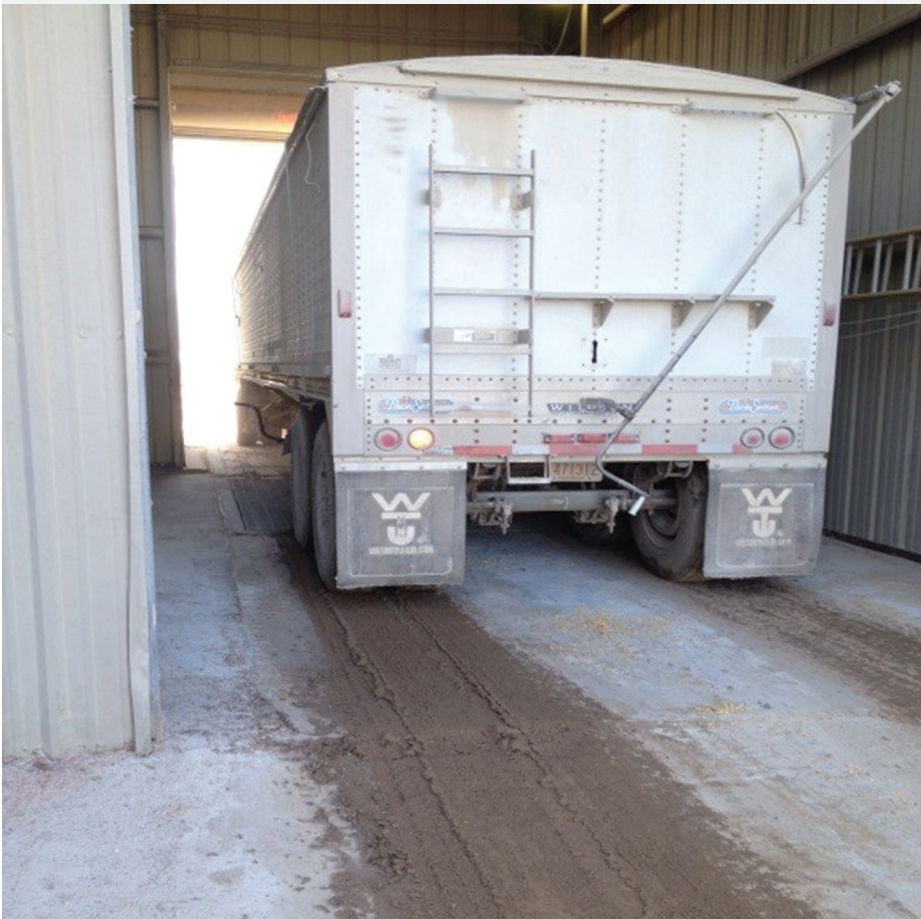
Figure 3: Example of potential contamination entering the dump pit by truck
