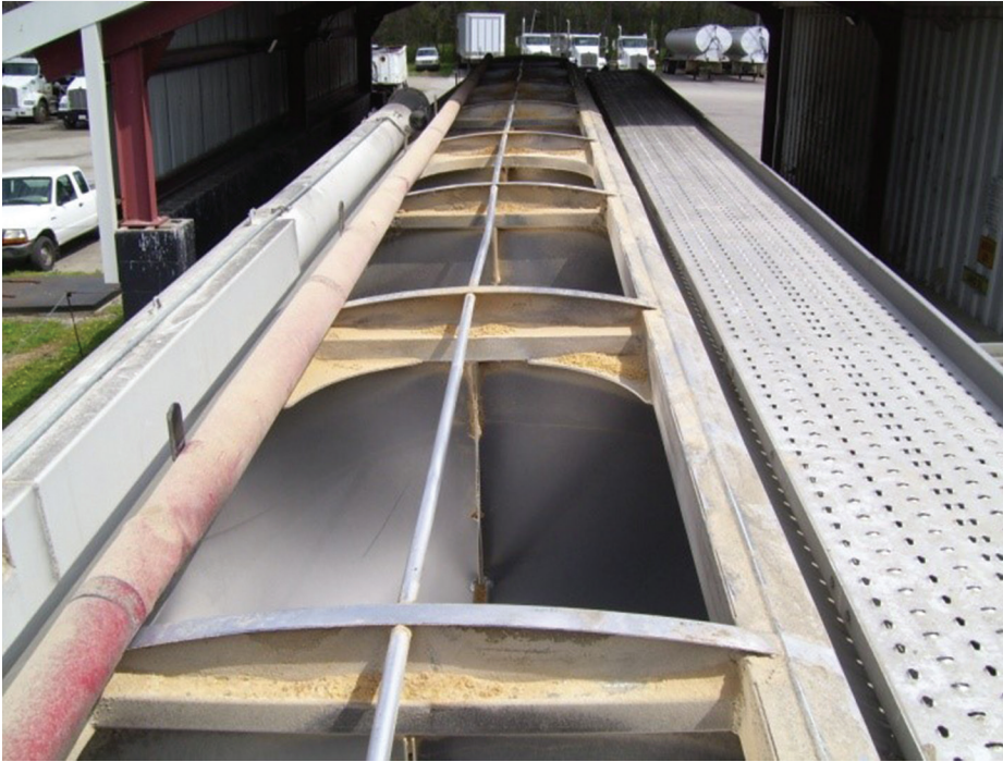
Figure 8: Potential contamination from leftover material in the top of a bulk feed truck
